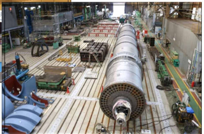
Steam tube dryer
